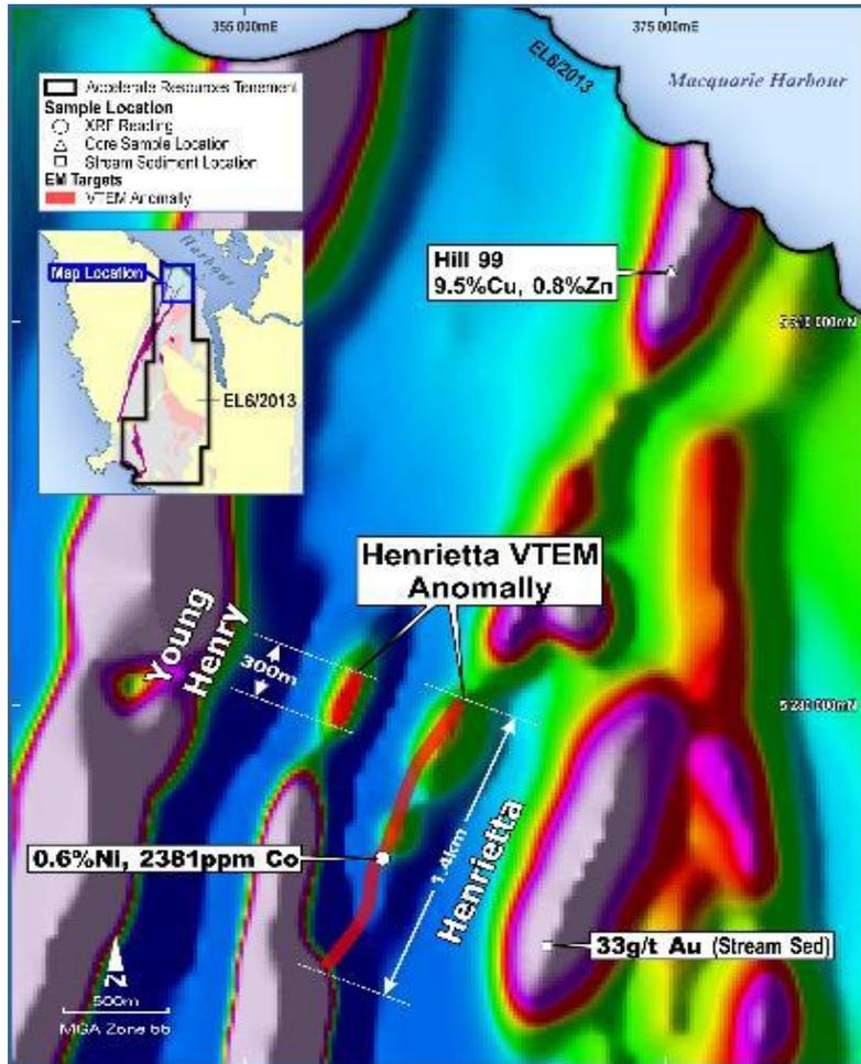
Figure 1: Location of Young Henry and Henrietta airborne electromagnetic (VTEM) anomalies over aeromagnetics with ultramafics and faults highlighted.
