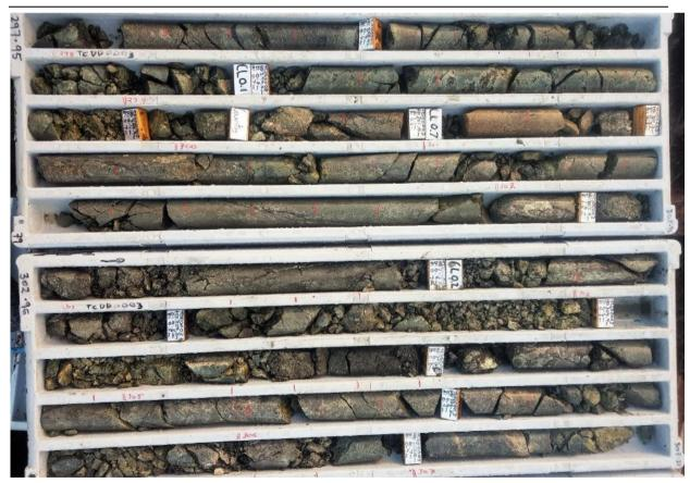
Photo 1: Drill Core TCD003 297.95m to 307.31m
