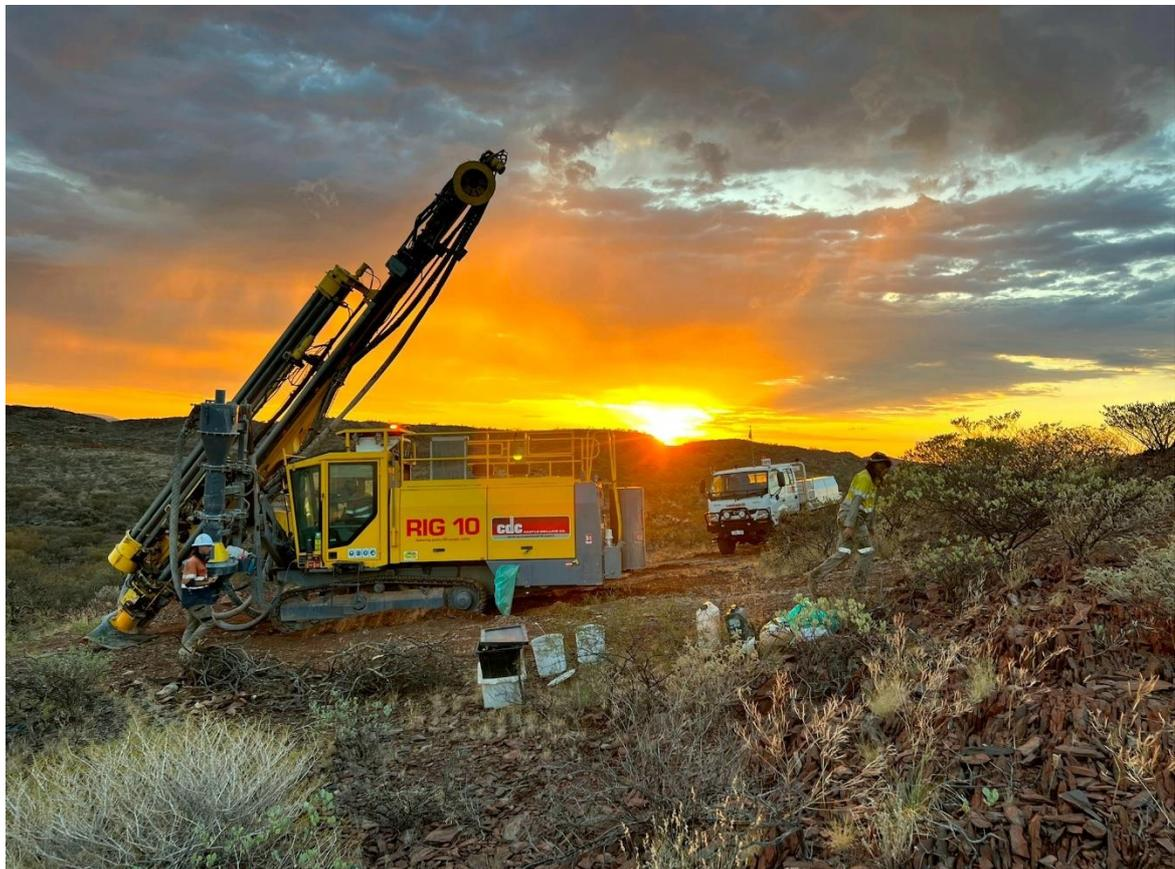
Figure 1: Track-based RC rig onsite and ready for action
