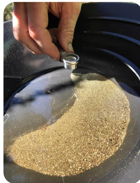
*panned pyrite-chalcopyrite sulphides + gold from saprock ore*
