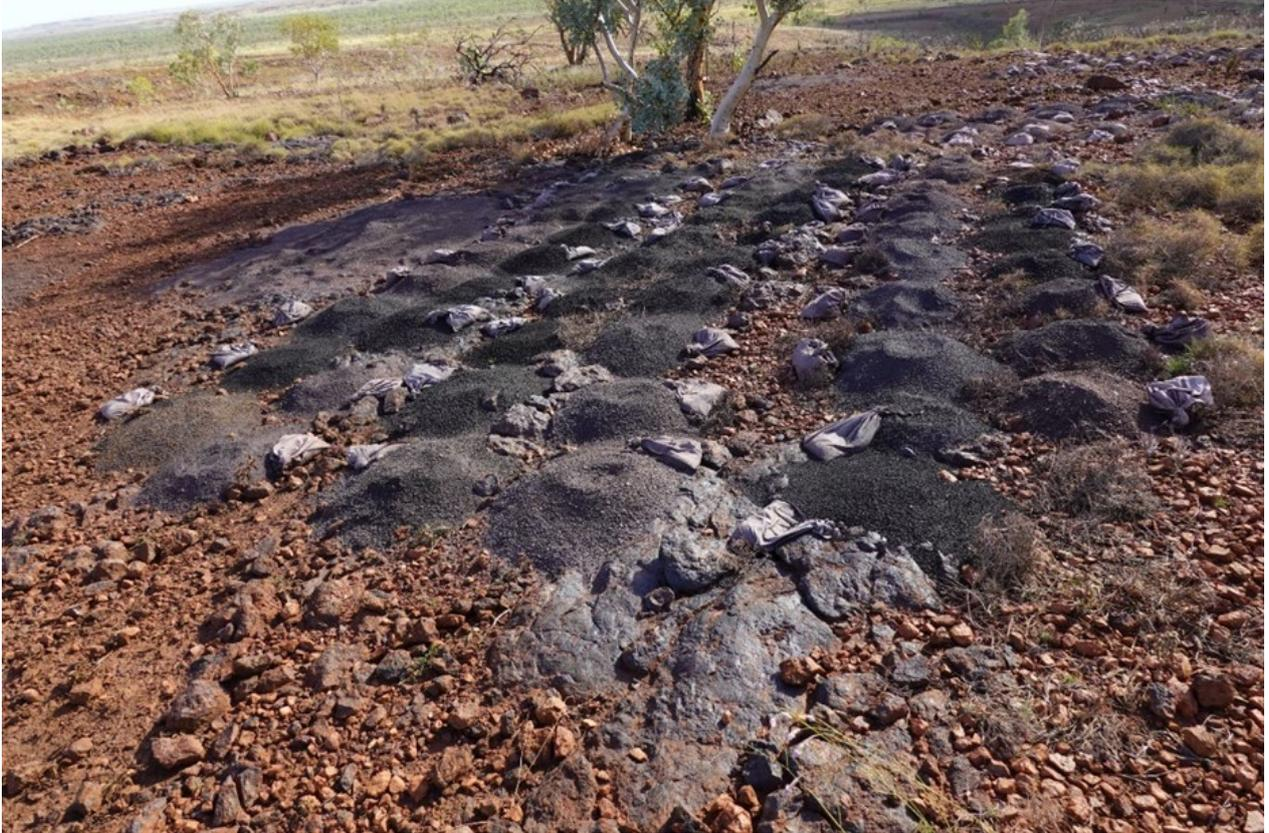
Figure 14. Photo of RC chips from drill hole WNRC089 at Nathan's Flat in Area 42.
