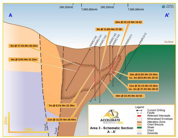
Figure 5 – Geological cross section of Barra South Area 3 showing significant intercepts.
