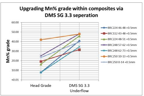
Figure 2 - Chart showing upgrade of manganese composite samples by DMS.
