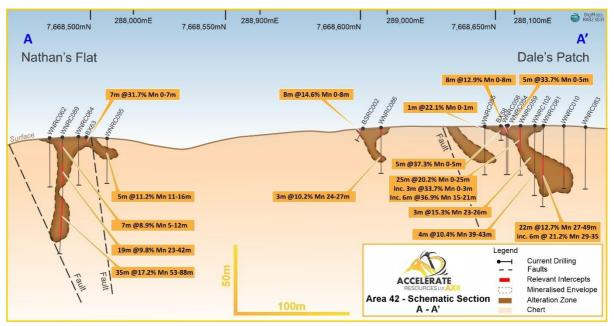
Figure 7 – Geological cross section of Area 42 showing significant intercepts.
