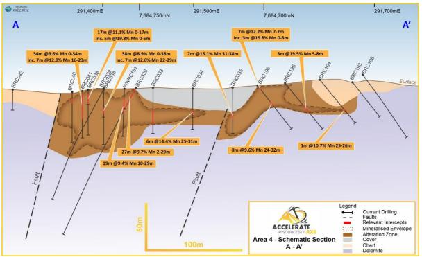
Figure 6 – Geological cross section of Barra South Area 4 showing significant intercepts.
