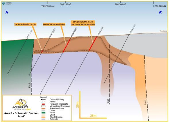
Figure 4 – Geological cross section of Barra North Area 1 showing significant intercepts.
