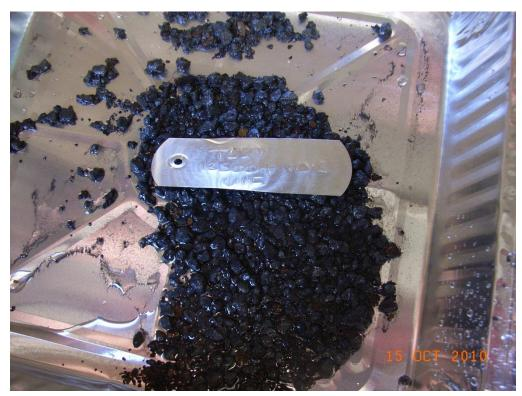
Figure 1: Photo from the 2010 DMS beneficiation test work showing Mn concentrate
