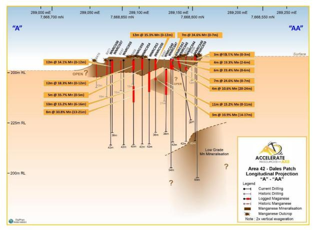
Figure 3 - Dale's Patch Long Section
