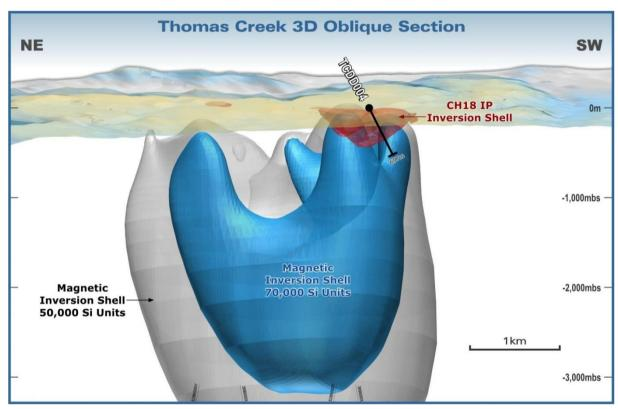
Figure 2: IP chargeability and magnetic inversion shells targeted by TCDD004.
