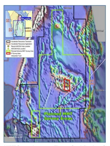
Figure 3. Proposed MMT Survey Areas over Thomas Creek Porphyry System on 1vd RTP
