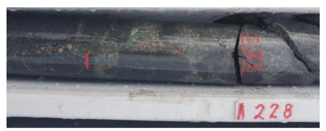
Picture 2: Strongly veined zone bearing actinolite
