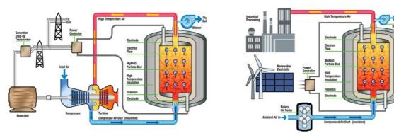
Figure 4 - RedoxBlox long duration energy storage technology for grid and industrial heat applications
