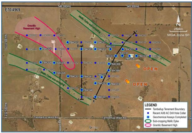
Figure 5: Sadlers prospect Location showing recent drilling and cross section lines on aerial imagery
