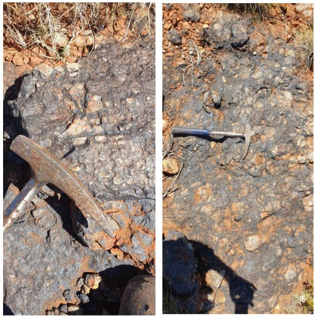
Figure 5: Manganese mineralisation as a matrix in the Pinjan Chert Breccia
