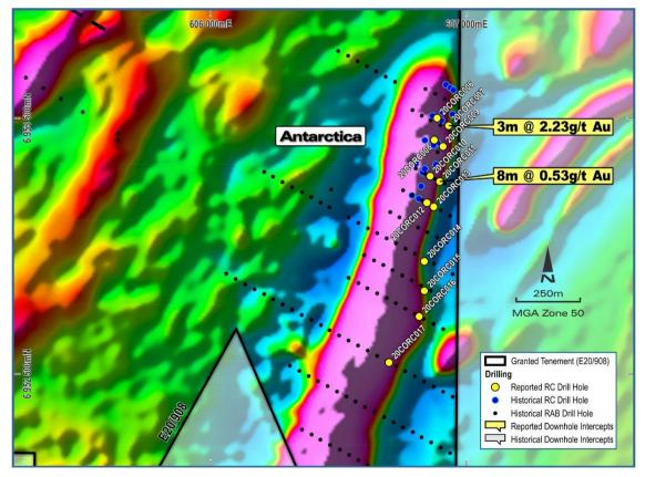
Figure 4. Antarctica Prospect. Drillhole locations and significant drill intersections over magnetics.
