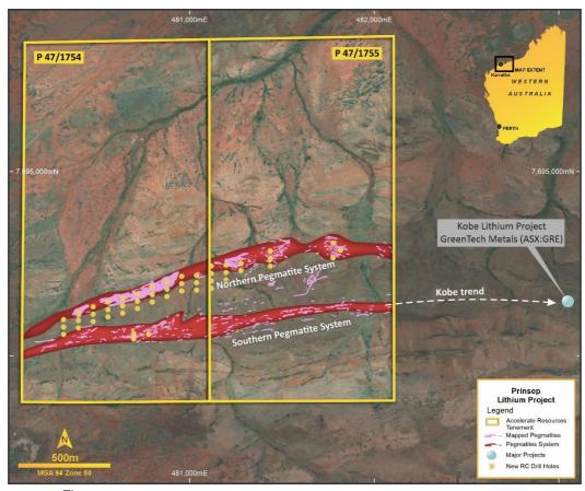
Figure 4: Proposed drill hole collar location for the Prinsep maiden drill program
