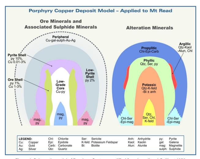
Figure 1. Schematic model of Porphyry System, modified from Lowell and Guilbert 1970
