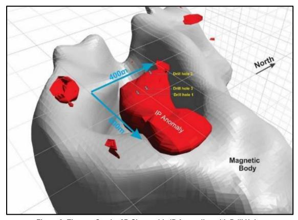
Figure 3: Thomas Creek - 3D Chargeable IP Anomalies with Drill Holes
