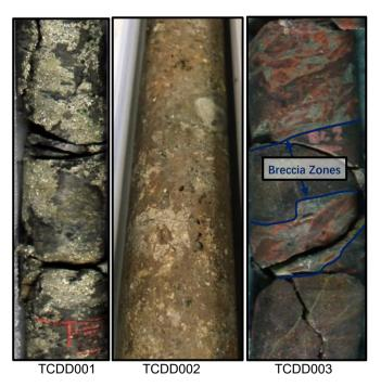
Photo 1. TCDD001, 150.7 to 151.05m, semi-massive to massive pyrite associated with anomalous cobalt assay results; TCDD002, 100.6 to 100.8m, semi-massive pyrite associated with minor zone of anomalous copper; TCDD003, 81.1 to 81.3m, Potassic Alteration in brecciated fault zone with associated disseminated pyrite.
